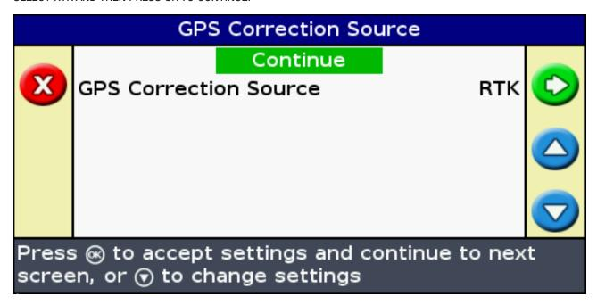
MAKE SURE TO SELECT TRIMBLE RADIO AND THE CORRECT NETWORK ID. NOW SCROLL DOWN TO SECURERTK KEYS AND PRESS OK.
