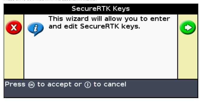
SELECT THE KEY YOU WISH TO ENTER AND THEN PRESS OK. EACH KEY WOULD REPRESENT A DEALER NETWORK. YOU MAY ENTER UP TO 5 DIFFERENT KEYS TO HAVE ACCESS TO 5 SEPARATE RTK NETWORKS.
