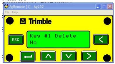
PRESS "V" UNTIL AT "KEY #1 KEY" SCREEN. CONFIRM CODE IS CORRECT. TO CHANGE CODE, GO TO "KEY #1 DELETE" SCREEN (ABOVE). PRESS "ESC" TO GO BACK TO HOME SCREEN.
