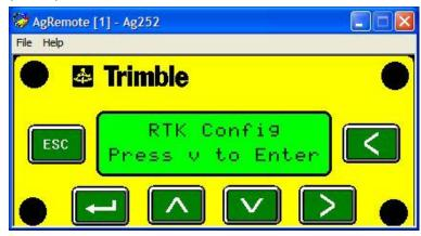
FROM "RTK CONFIG" SCREEN, PRESS "V" UNTIL AT "PRESS (BOTTOM-LEFT ARROW) TO ENTER SECURE RTK KEYS" SCREEN (BELOW)
