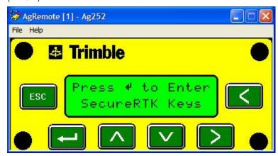
FROM "PRESS (BOTTOM-LEFT ARROW) TO ENTER SECURE RTK KEYS" SCREEN (BELOW), PRESS BOTTOM-LEFT ARROW UNTIL AT "KEY #1 KEY" SCREEN (BELOW)
