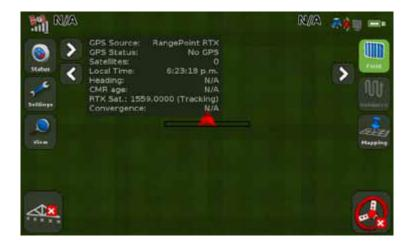
The GPS Source should show RangePoint RTX. GPS Status should show Converged. Convergence can take up to 5 minutes in a clear sky environment.
