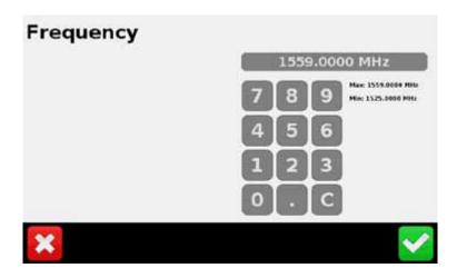
After you have entered the frequency, select the green checkmark button to return to the RangePoint RTX Satellite Settings screen. Select the Baud Rate button.
