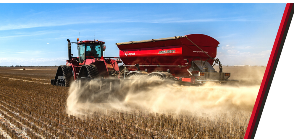
One of the test results captured by Fertilizer Australia, showing a 41m bout width.
